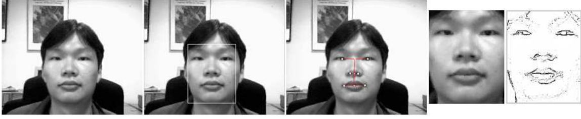
Fig. 5. (left to right): Sample test image; Detected inner face region; Extracted facial feature points and geometric measures; Normalized and cropped face; Face edges extracted from parameterized fuzzy edge detector.
