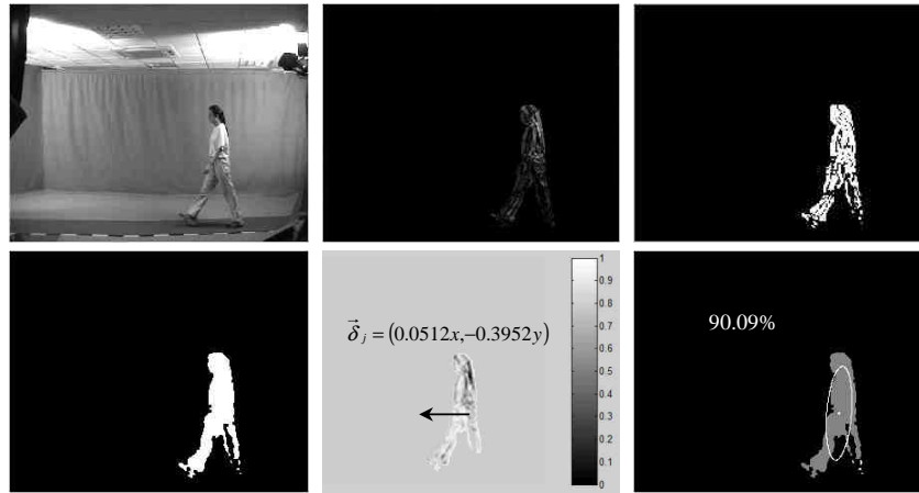
Figure 3 – A sample sequence from the Southampton Human ID database showing various stages of the proposed algorithm; original frame with motion of a person walking (top left); adjacent frame subtraction (top middle); motion image (top right); motion image after preprocessing (bottom left); motion vector \vec{\delta}_j (bottom middle); and ellipse fitting (bottom right).
